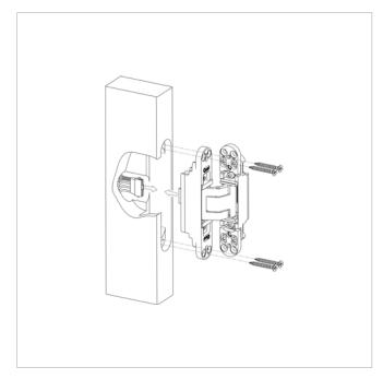
Sharp edges should be avoided in the cable feedthroughs to protect against cable damage. Conduct additional routing on both sides for the cable feedthrough. Establish the plug connection and mount the door part.
